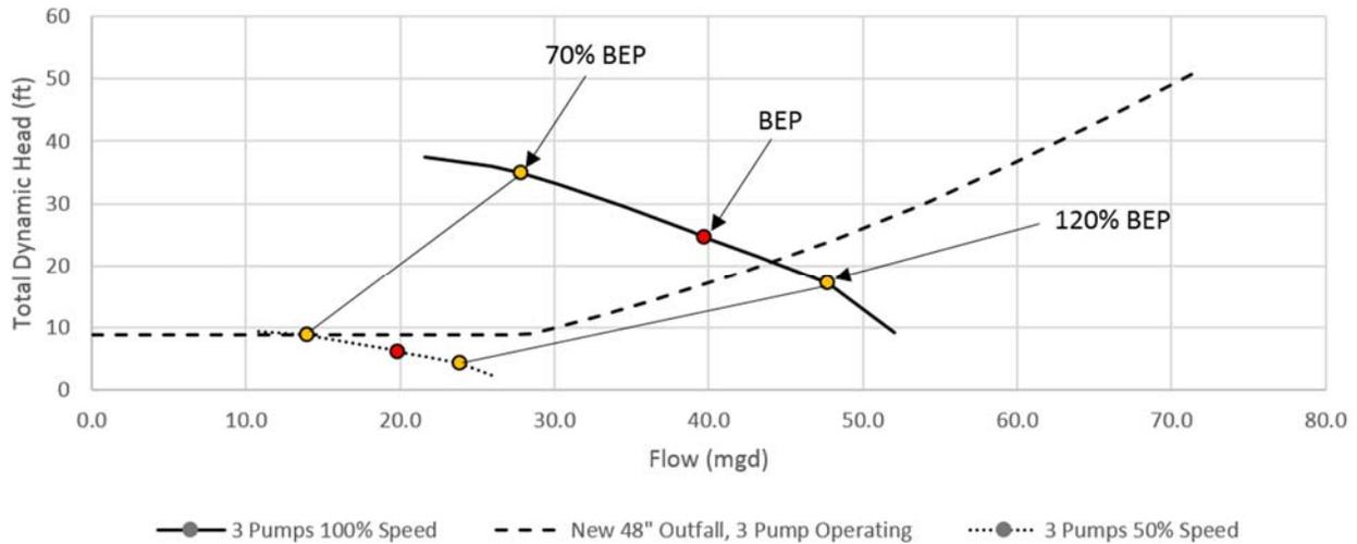
**Figure 10. Three Pumps Operating**
