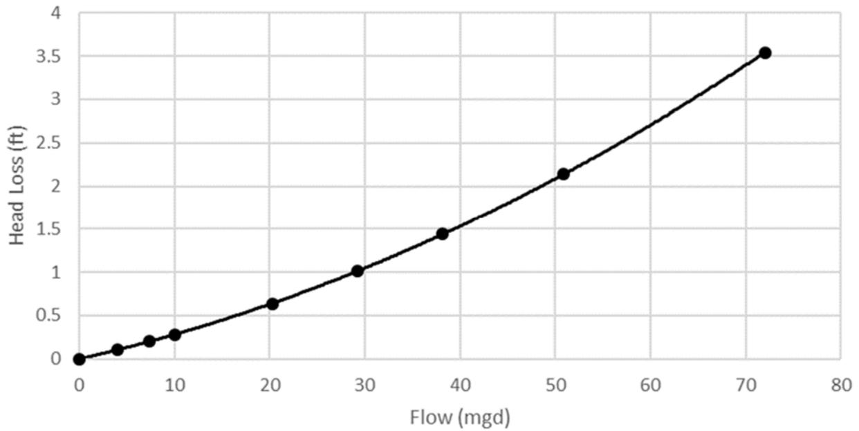
Figure 4. Diffuser and Manifold Head Loss
