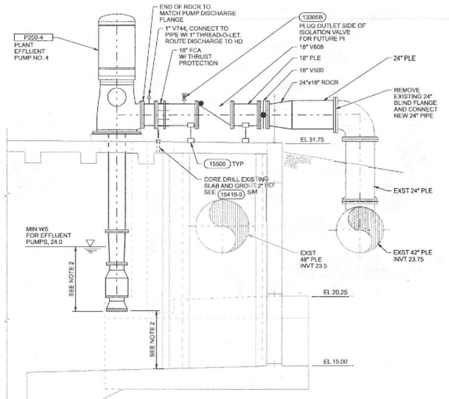
Figure 2. Effluent Pump Station Configuration Section
