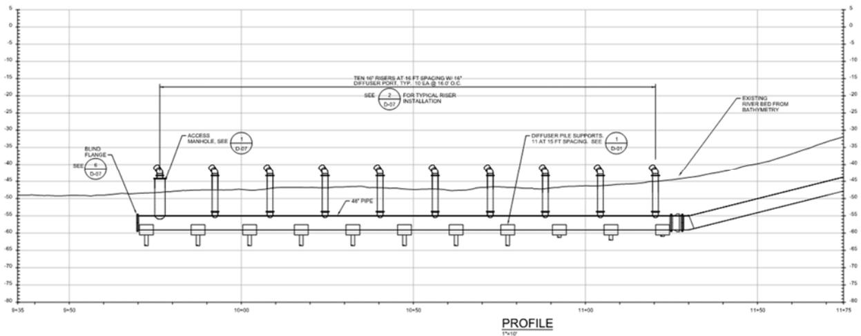
**Figure 3. Diffuser and Manifold Configuration**
