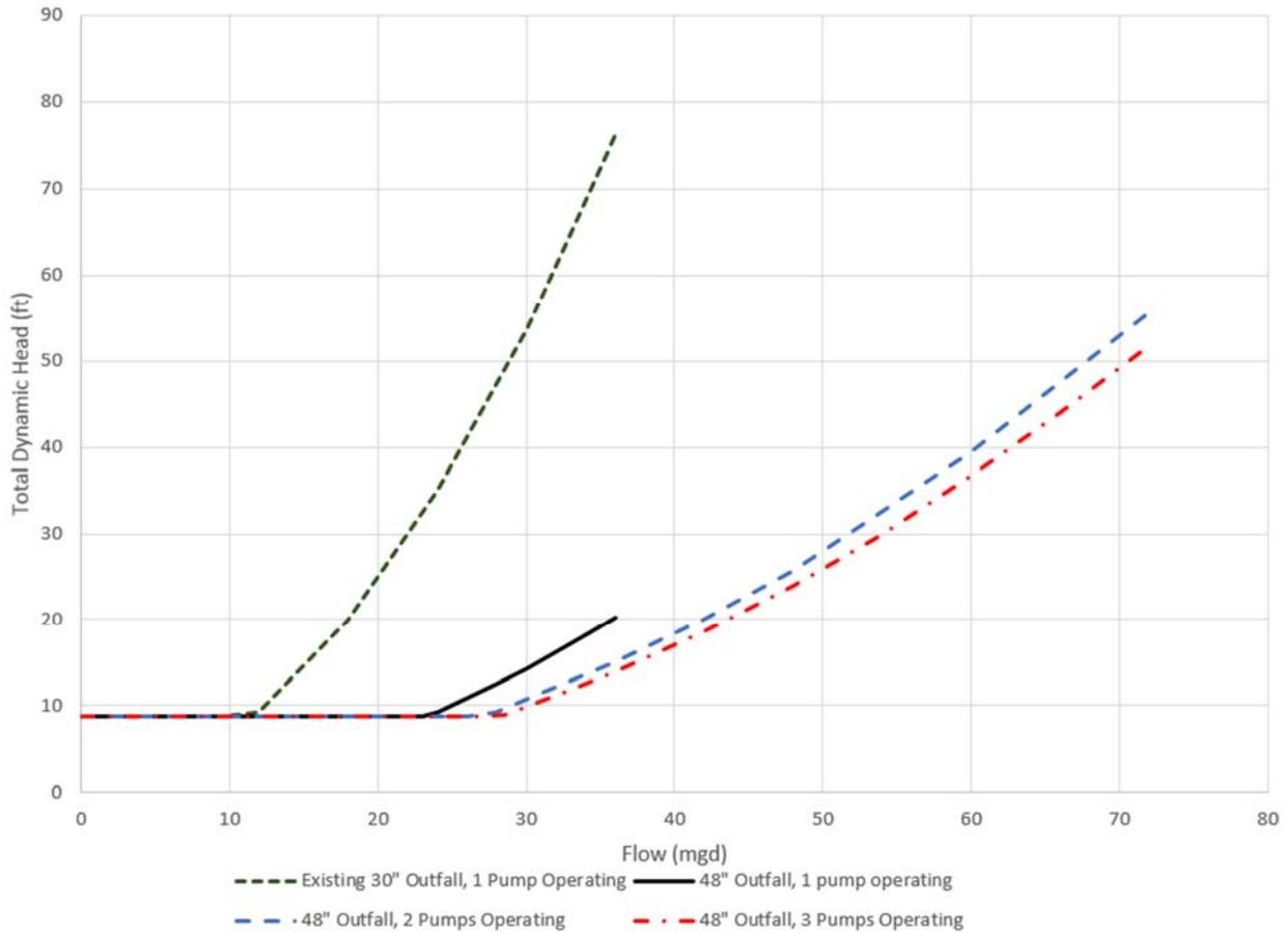
Figure 7. System Curves, New 48-Inch-Diameter and Existing 30-Inch-Diameter Pipelines
