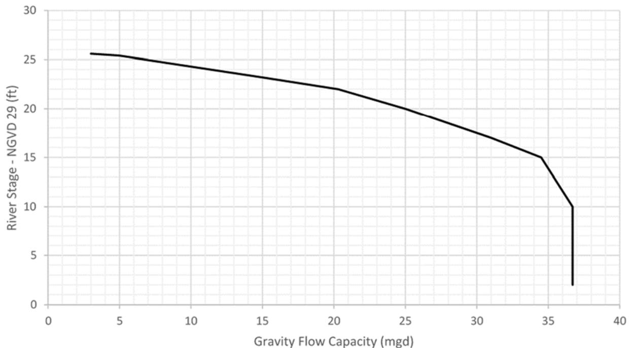
Figure 5. River Elevation versus Allowable Gravity Flow
