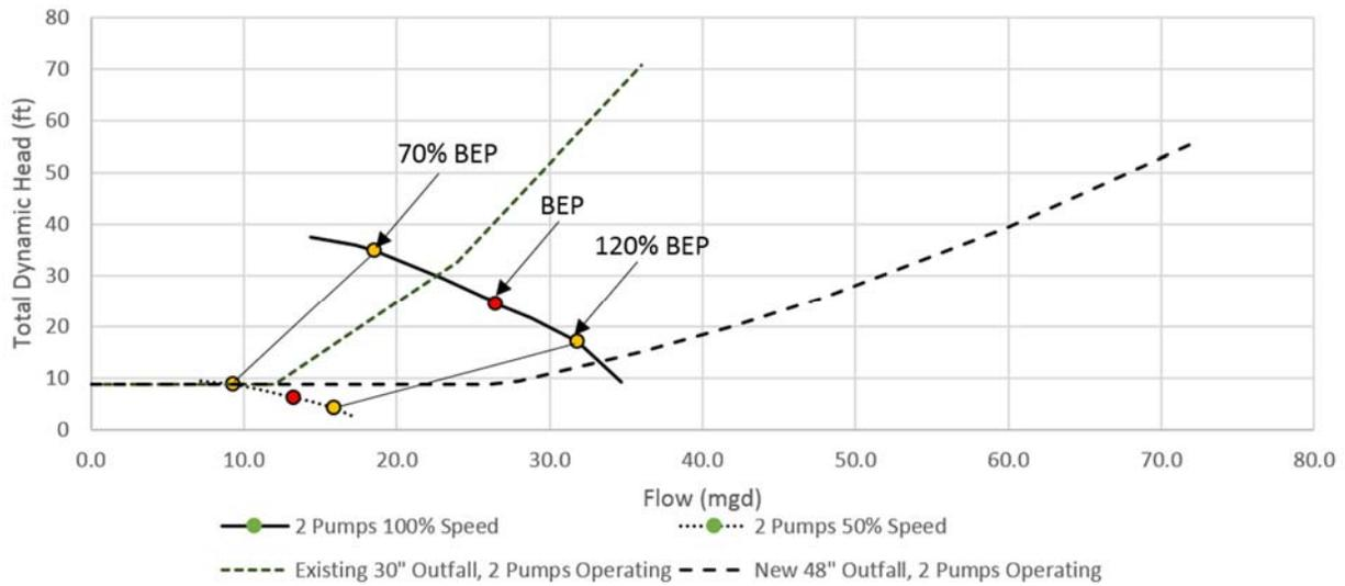
**Figure 9. Two Pumps Operating**
