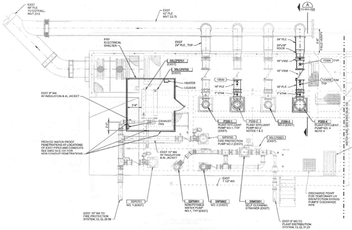
Figure 1. Effluent Pump Station Configuration Plan
