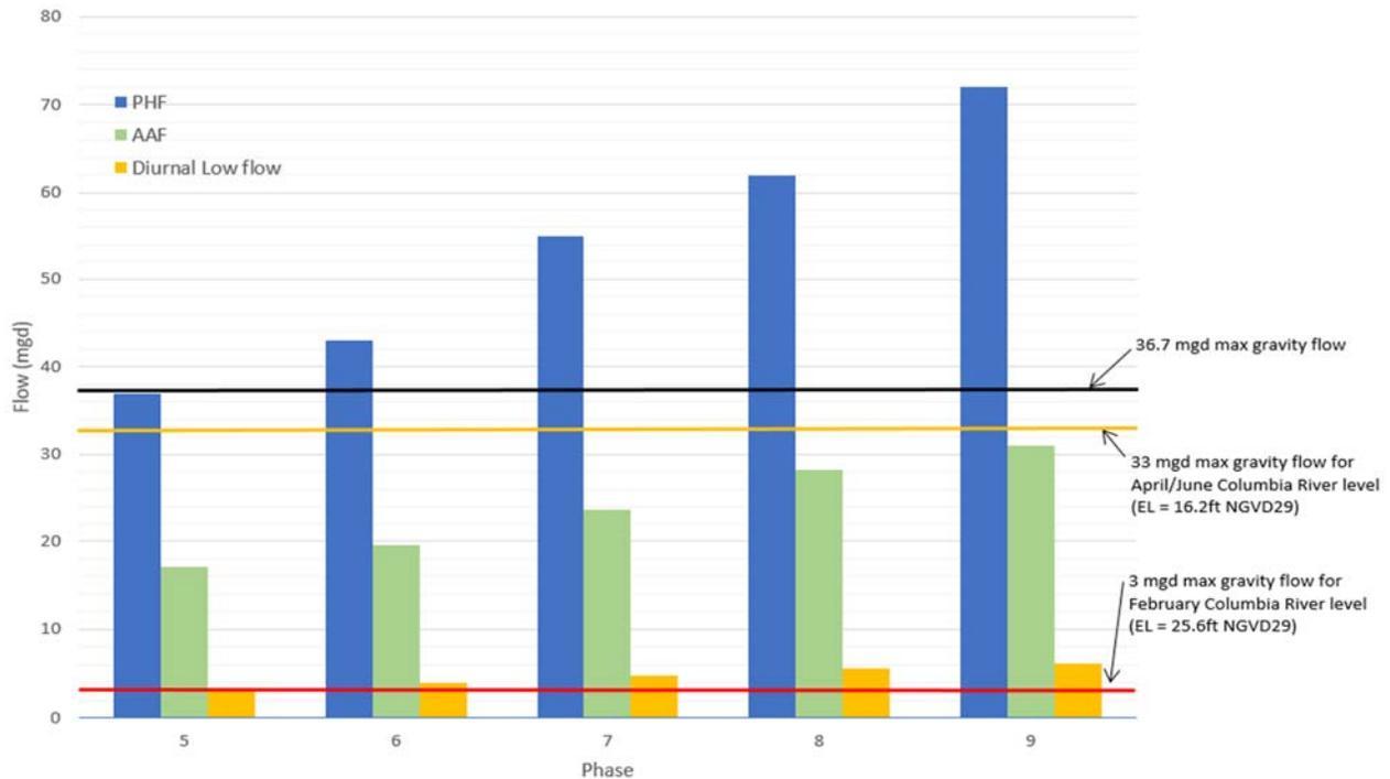
Figure 6. Effluent Flow by Phase with Gravity Flows at a Variety of River Elevations
