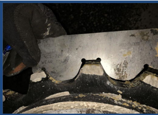
Tooth Wear on Existing NCS-720S Idler Sprockets
