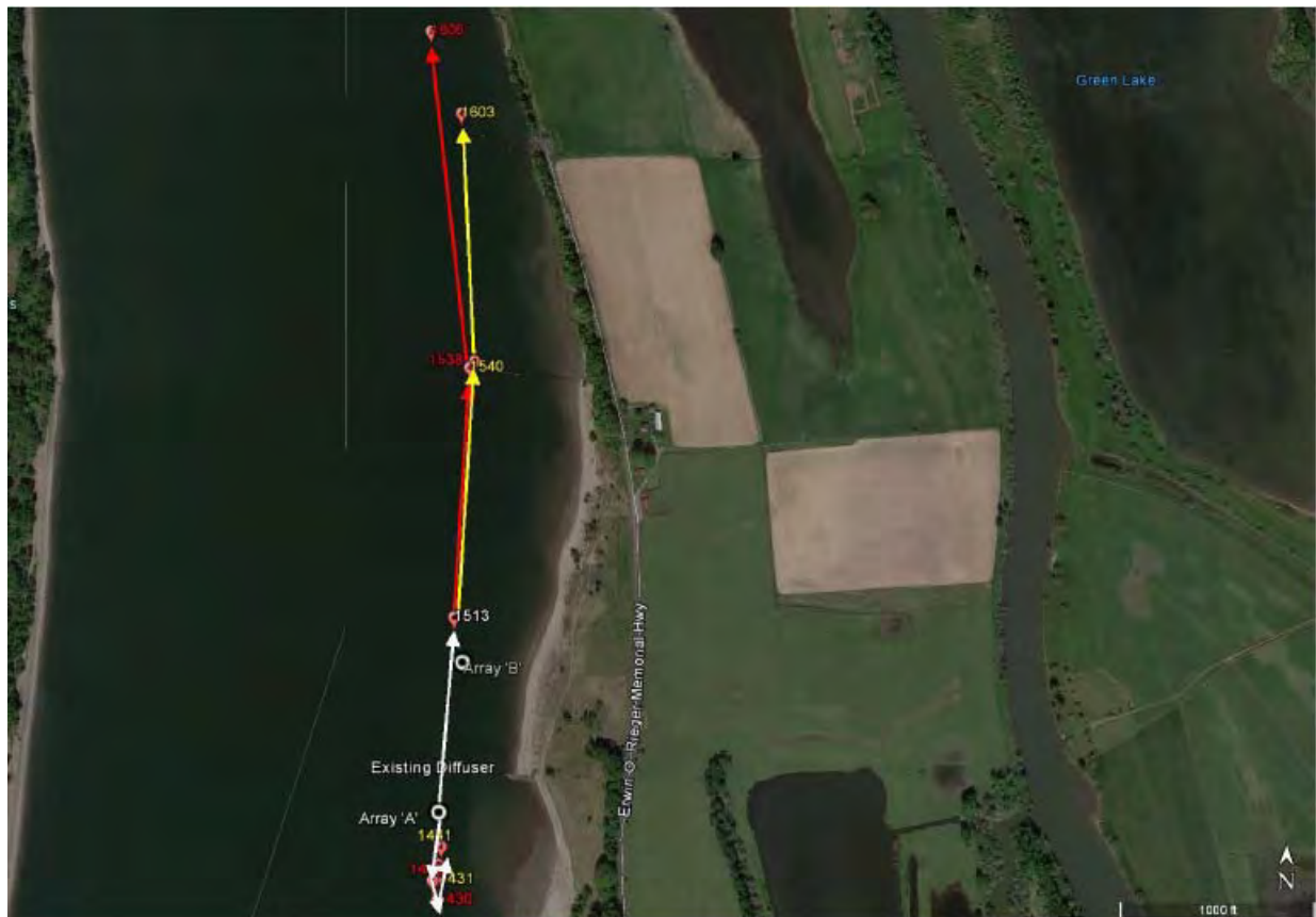
Figure 2-11. Probable Discharge Plume Trajectory Plot from Drogues Released at Potential Diffuser Site 1 (Array A) near Columbia River Mile 96 on September 23, 2015
