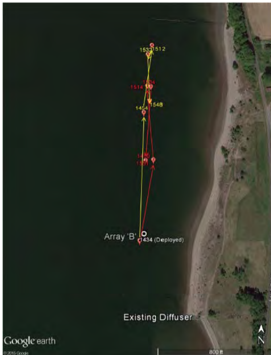
Figure 2-12. View of Probable Discharge Plume Trajectory Plot from Drogues Released at Potential Diffuser Site 2 (Array B) near Columbia River RM 96 on October 14, 2015
