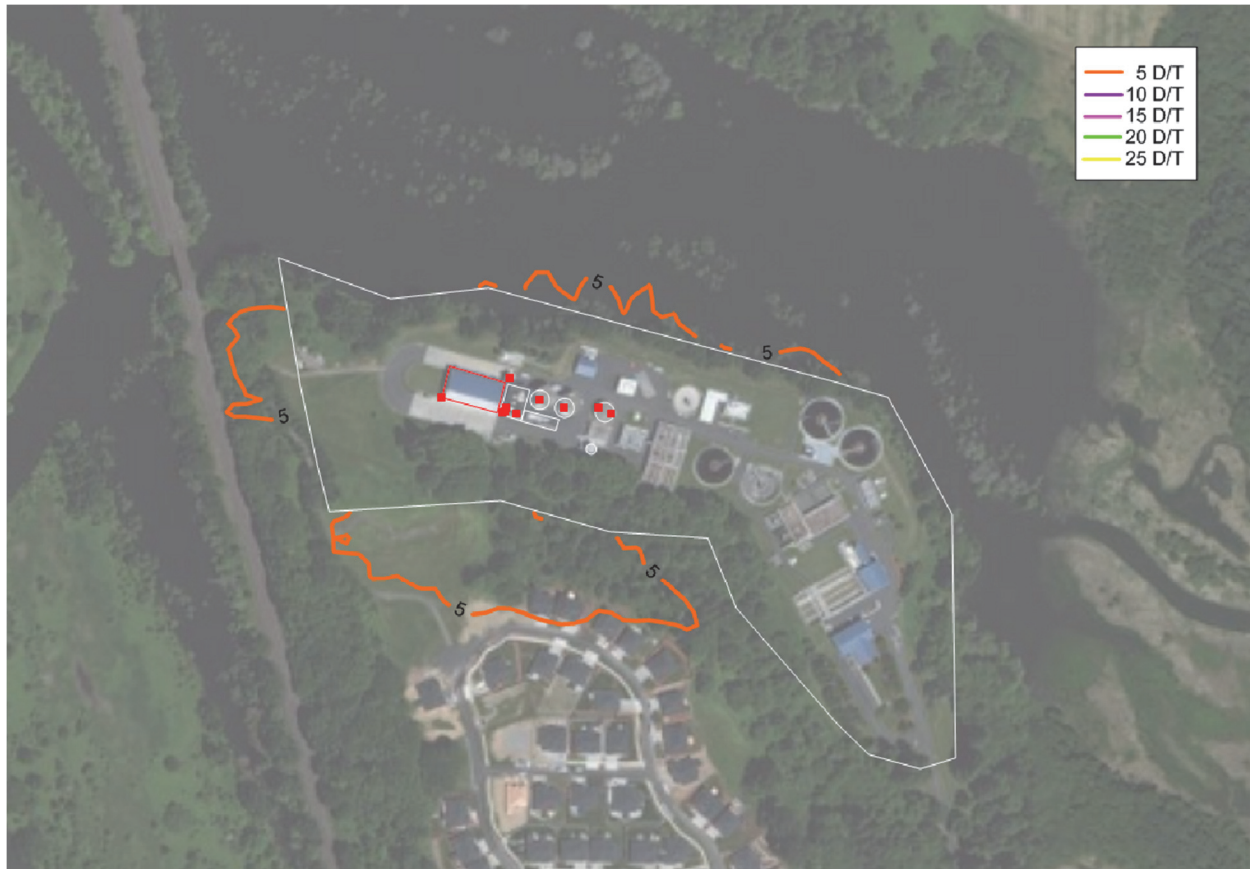
Figure 3-5. 1-Hour Annual Average Isopleths Showing Lines of Constant Odor Concentration in D/T—Overall Solids Area with Major Odor Sources Treated
