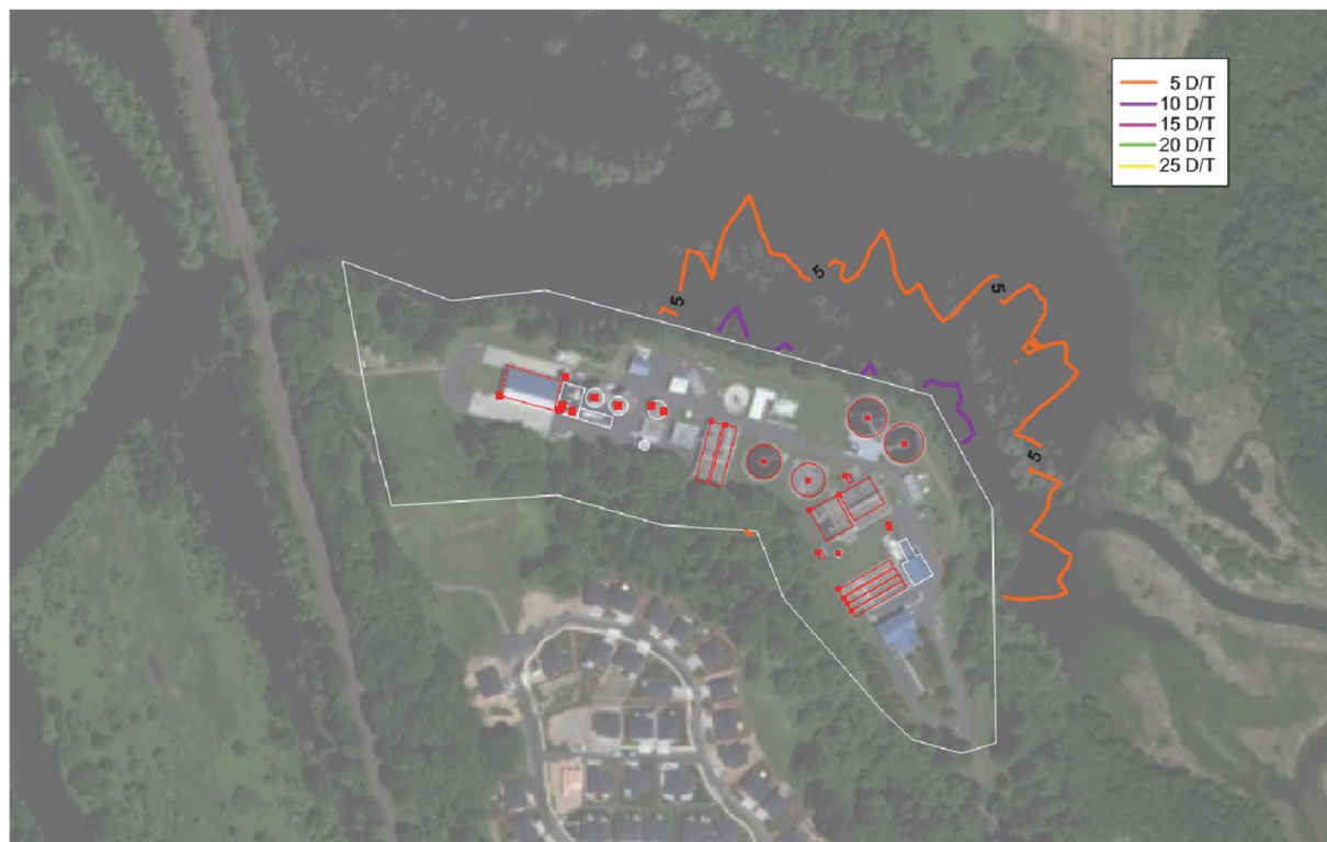
Figure 3-1. 1-Hour Annual Average Isopleths Showing Lines of Constant Odor Concentration in D/T—All Liquids Odor Sources with Odor Control as Proposed in Phase 5B Improvements
