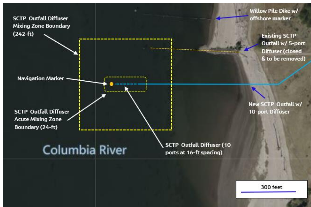
Figure ES-3. Schematic Illustration of SCTP New Outfall Diffuser Location and Acute and Chronic Mixing Zone Boundaries in the Columbia River
