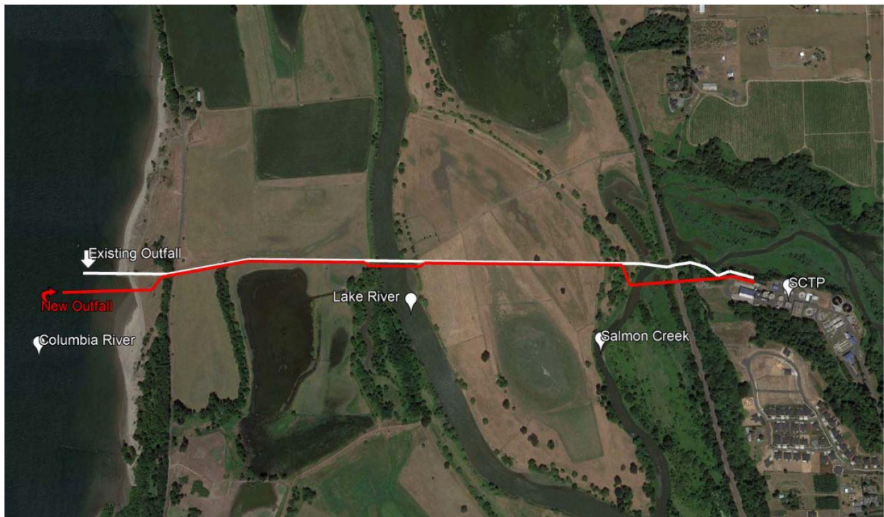
Figure 1-1. Overview of SCTP, Existing 30-inch and New 48-inch Effluent Pipelines, and the Location of the Original and New Outfall Diffusers in the Columbia River
