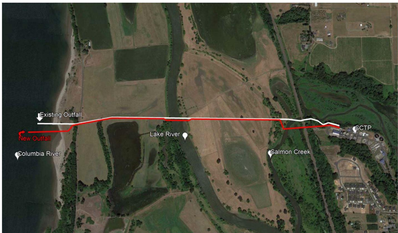
Figure ES-1. Overview of SCTP, Existing 30-inch-diameter and New 48-inch-diameter Effluent Pipelines, and the Location of the Original and New Outfall Diffusers in the Columbia River
