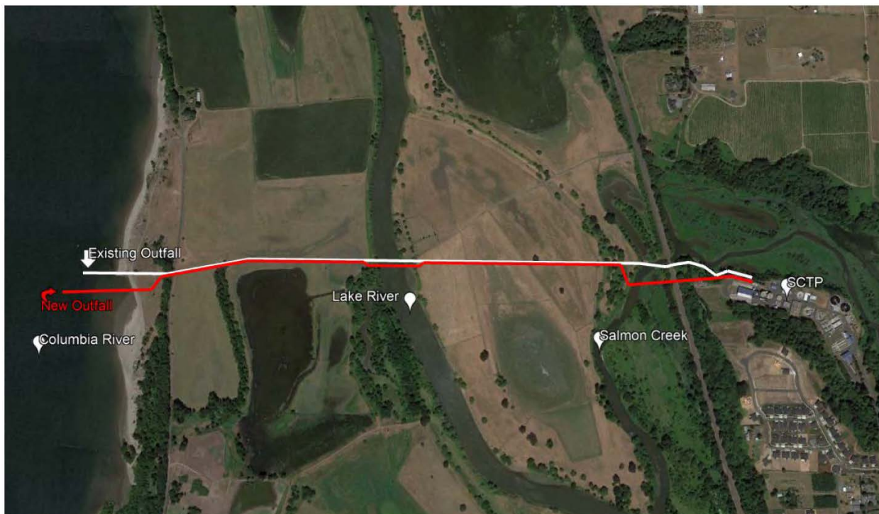
Figure 1. Overview of Salmon Creek Treatment Plant, Existing 30-inch and New 48-inch Effluent Pipelines, and the Location of the Original and New Outfall Diffusers in the Columbia River
